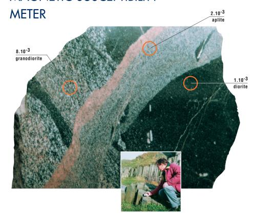
The SM-20 magnetic susceptibility meter is useful for a number of geological and geophysical applications where the unique sensitivity of 10<sup>-6</sup> SI units together with its small, shirt-pocket size and light weight are appreciated.
