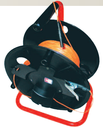
Potential Cable Reel
